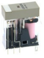
G2R-2-S 110VAC (S) Relay, plug-in, DPDT, 5 A, mechanical indicator, 110 VAC
