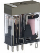
G2R-2-S 230VAC (S) Relay, plug-in, DPST, 10 A, mechanical indicator, 230 VAC
